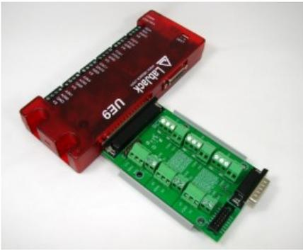
Figure 2: Connected by P2 - DB37 Connector
