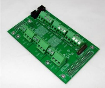
OEM PS12DC boards are useful for direct solder applications, when the functionality is already understood, and the device can be incorporated without the easy-to-use connectors.
