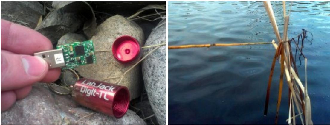
The Digit-TLs were configured to log temperature at a 10 minute interval, and each was equipped with a rugged aluminum enclosure.
