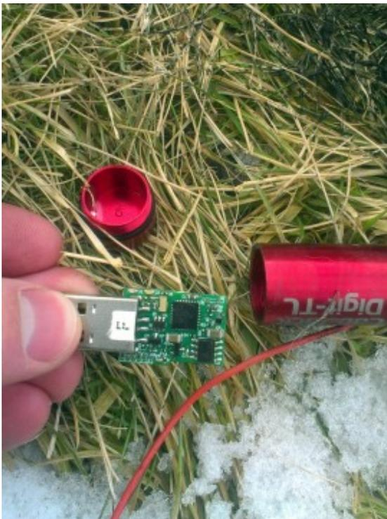
The case is totally dry inside, definitely a comforting sign. It's important to fully submerge this case because the O-ring can dry out in the sun and crack - leading to eventual leaks. When pulling these out of the water, make sure your hands are dry before touching the device directly.
