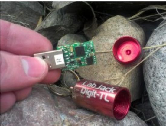
The case was faded due to exposure to the sun, but nothing too bad. The O-ring had some cracks, but seems to be watertight enough to keep moisture out. This O-ring is probably too cracked for full submersion in water now, which is why we provide extra O-rings with each Digit-TL aluminum enclosure.
