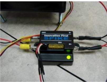
Shown is an old Spike motor controller that was lying around, but any digitally controlled H-Bridge capable of the current draw through the peltier would have worked. Wire the PSU to the input lines, and the peltier on the M- M+ lines. Connect the digital control wires to any of the Labjack U3 FIQ (Flexible Input Output) terminals.
