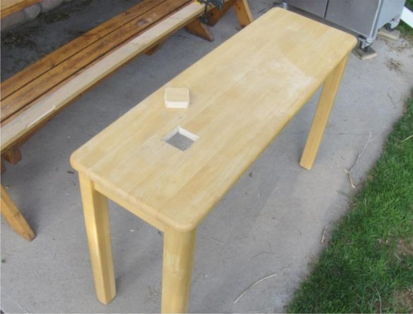
Cut an opening using a drill and a reciprocating saw. Make sure the peltier and insulation can fit through.
